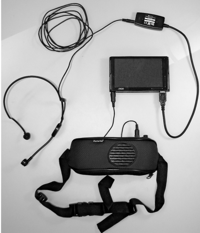
Figure 1. BioSpeech system components: Headset (left) is attached via USB adapter to PC (middle, belt attachment not shown), which is attached to amplified speaker (bottom, with adjustable belt).
